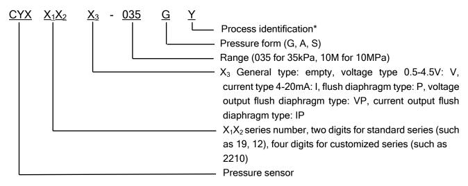
\*Process identification: f for general process, Y for negative pressure process.
