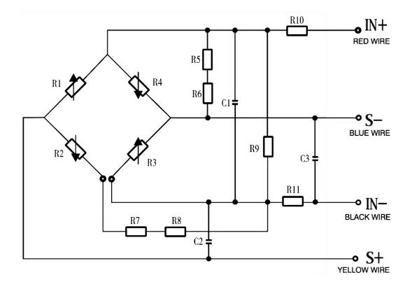
IN + (red wire) - power supply positive S + (yellow wire) - output positive IN - (black wire) - power supply negative S - (blue wire) - output negative
